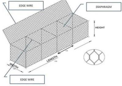
Figure 5 The regular assembly of the wire mash cages [11]
